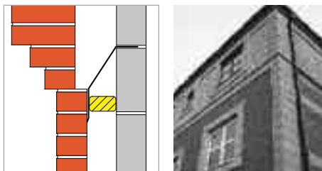
Cavity dropcloaks protect high-level dentil coursing and intermediate strings. The masonry bonding of the exterior skin is not interrupted. (1752)
