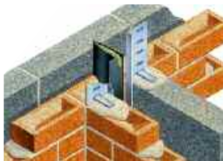
Original exterior wall becomes an interior wall when an extension is constructed. Vertical DPC integrity is required as well as horizontal DPC integrity.
