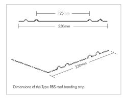
Produced to an overall width of 230mm, the Type RBS is fire resistant in accordance with BS 476, the classification being to P60 (SAB) class three.
