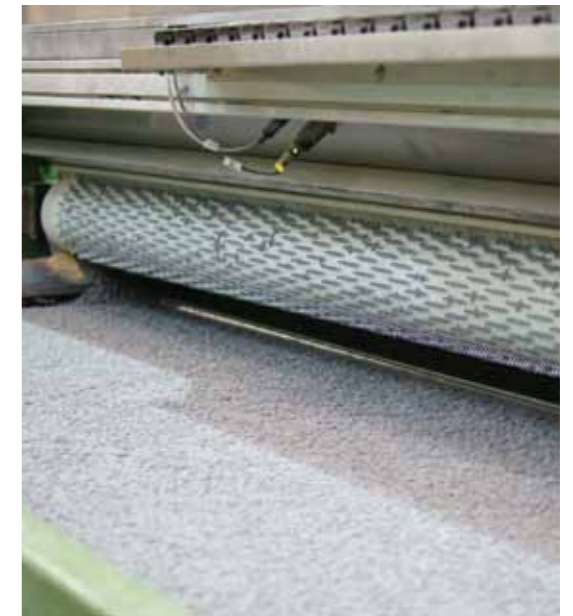
Recycled tile backing being produced at our Ripley plant
