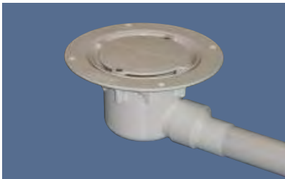
Connecting to 43mm (1 1/2") ABS. Use 50mm (2") to 43mm (1 1/2") solvent cement reducer (provided).
