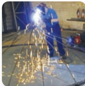
The gazebo under construction in our Manufacturing works.
