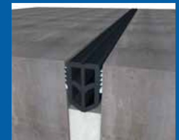
Newton 305 ActiveJoint This water bar has a unique 'V' shape with a number of barbs, creating more grip as water pressure increases
