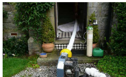
Full testing of Newton PAC System - remarkable results, Radon levels down from 5000 bq/m to 100 bq/m
