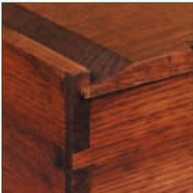
Detail of drawer traditional construction showing solid base and 'through' dove tail joints.
