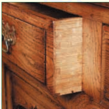
Detail of drawer showing fielded drawer front with dovetails and pierced back plate brassware.
