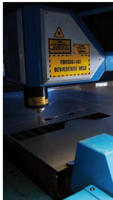
Stainless steel being cut with a laser in the Danish factory
