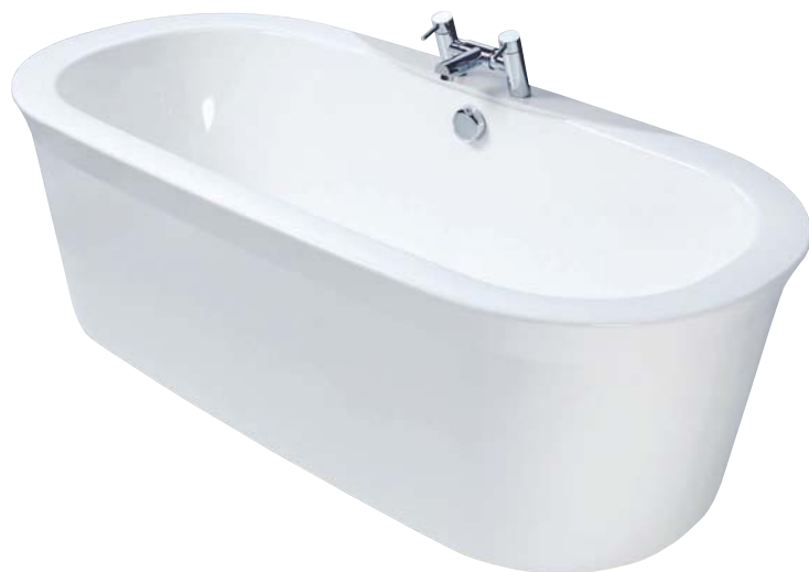
With tap deck and bath filler, no plinth. Note that if a 3 hole bath mixer is to be used then the bath should be ordered with the overflow to be on the opposite side to the tap deck, and an extended waste/overflow used.
