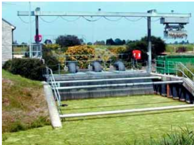
An Overhead Trashrake with curved track on a hydro-electric power station.
