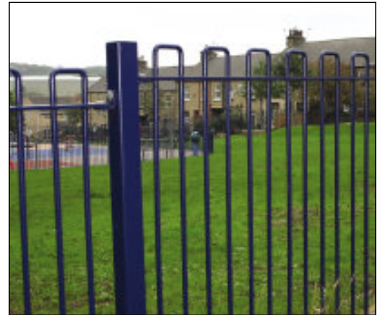
TITTESWORTH BOW TOP Heights: 1000, 1200, 1400, 1600, 1800 and 2000mm. Post centres: 2.8m max. Infill bar size increases with height of fence.
