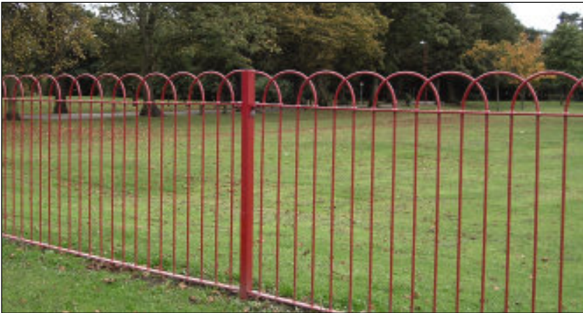
INTERLACED BOW TOP Heights: 600, 900, 1000, 1200, 1400, 1600, 1800 and 2000mm. Post centres: 2.8m max. Infill bar size increases with height of fence.
