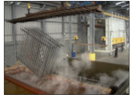
In house galvanising plant
