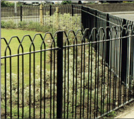
BLYTHE BOW TOP Heights: 1000, 1200, 1400, 1600, 1800 and 2000mm. Post centres: 2.8m max. Infill bar size increases with height of fence.
