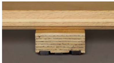
Rubber strips with maximum load (note that the outer strips are never squeezed to destruction thanks to the centre strip and their recessment).
