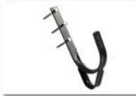
Trapac<sup>®</sup> Safety Hooks are for fixing loads such as roofers' ladders in place while work is being carried out on the roof. They are available in three versions to suit slate and profiled concrete and clay tiles and plain tiles. Safety equipment can also be hung on the eyelet.
