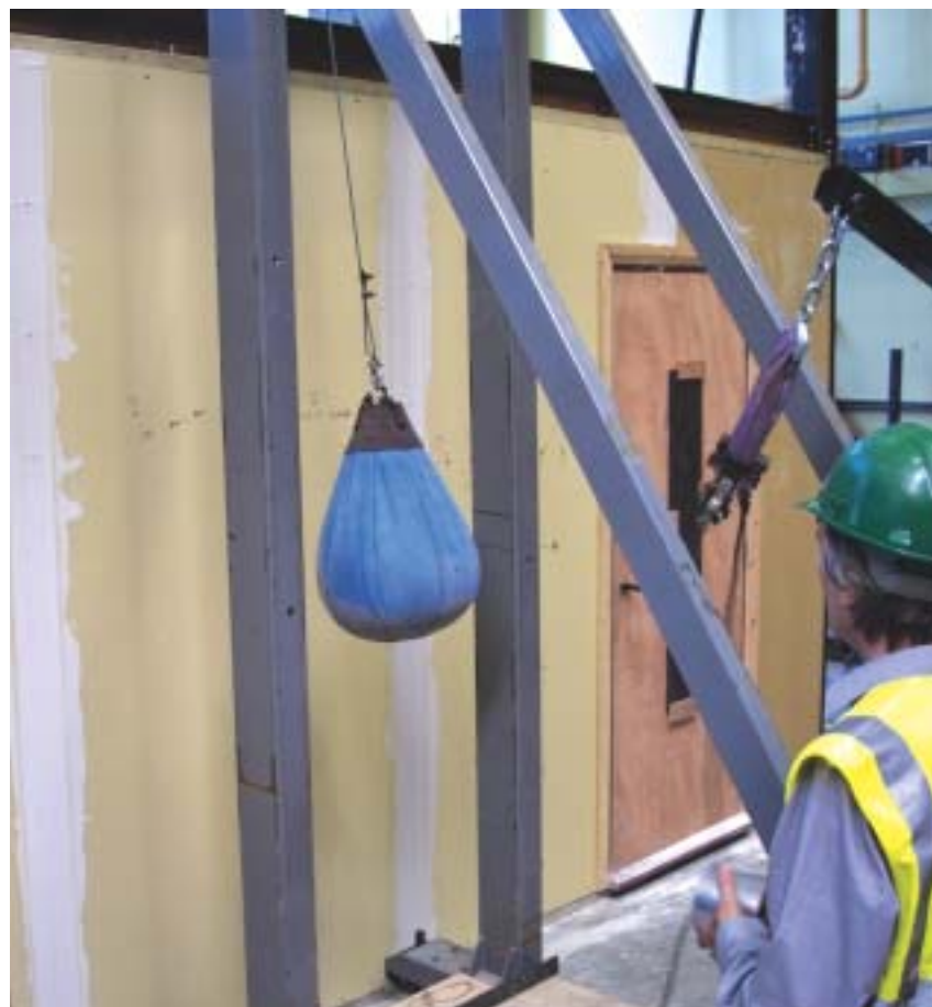
Above: BS 5234 Impact test being carried out at BRE Testing Centre
