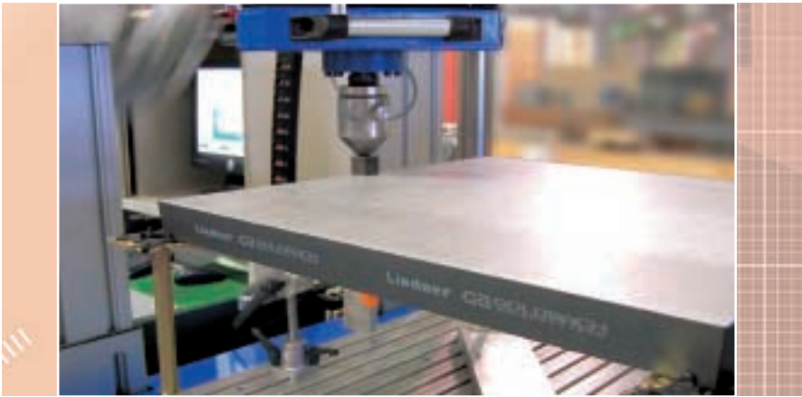
Inspection for load-bearing capacity
