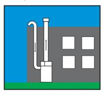
Vertical Balanced Flue Flues vertically using IGE/UP/10 approved flue material. Directly draws combustion air with
