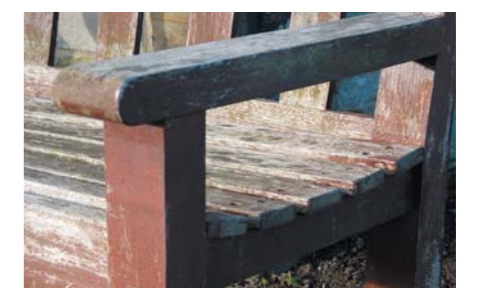
Traditional timber outdoor furniture exposed to wind and rain requires ongoing maintenance of painting or staining.
