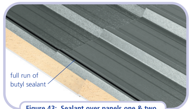
Figure 43: Sealant over panels one & two
