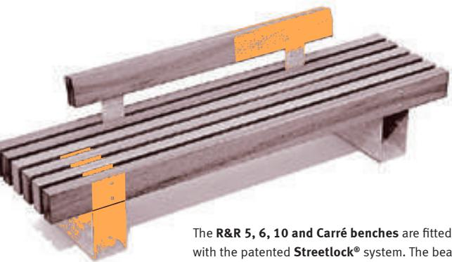
The **R&R 5, 6, 10 and Carré benches** are fitted with the patented **Streetlock®** system. The beams are not screwed, but locked with a stainless steel bar and theft-proof nuts. This construction allows the beams to be turned over or easily replaced. Very convenient in the event of damage!
