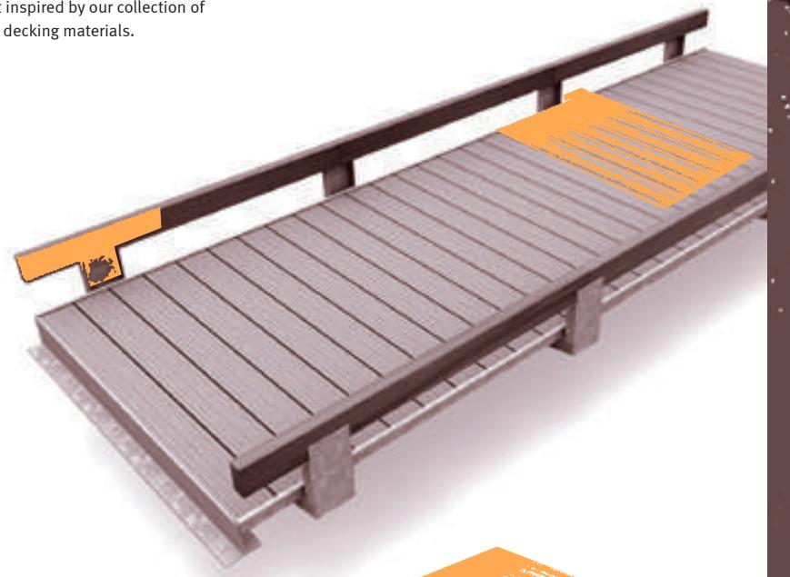
The **Country Bridge** is a flat bridge for bicycles and pedestrians. Minimal in design with a maximum span of 10 meters / 33 ft. The low and high R&R balustrades have industrial supports in galvanized or CorTen steel.
