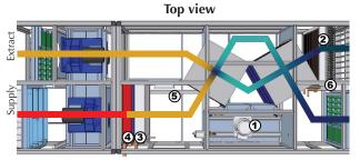
In night time mode the unit modifies the operating settings to adapt to the changes of evaporation from the pool and reduce consumption to the minimum.
