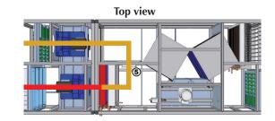
The operating mode is with no external air flow. The whole air flow is recirculated through damper 5 and returned to the pool area.
