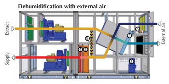
The operating mode is with external air dehumidifying the space, compensating for evaporation from the pool. The refrigerant circuit (consisting of the compressor 1 and the coils 2 and 3) allows the sensible and latent heat recovery of the extracted air to be transferred to the supply air or the water, through the thermal heat exchange consisting of the double heat exchanger on the water side.
