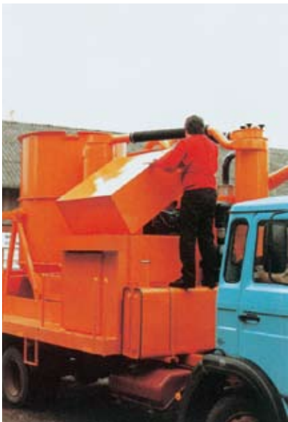
Aerzen bulk vehicle blower GM 13.f7-1 used on a mobile milling and mixing installation ▶ ▼
