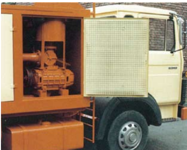
▲ ◀ Aerzen bulk vehicle blower GM 13.f7-1 used on a mobile milling and mixing installation producing feed
