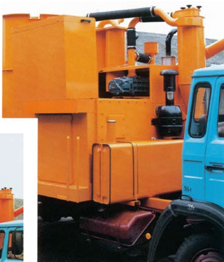
Aerzen bulk vehicle blower GM 13.f7-1 used on a mobile milling and mixing installation ▶ ▼
