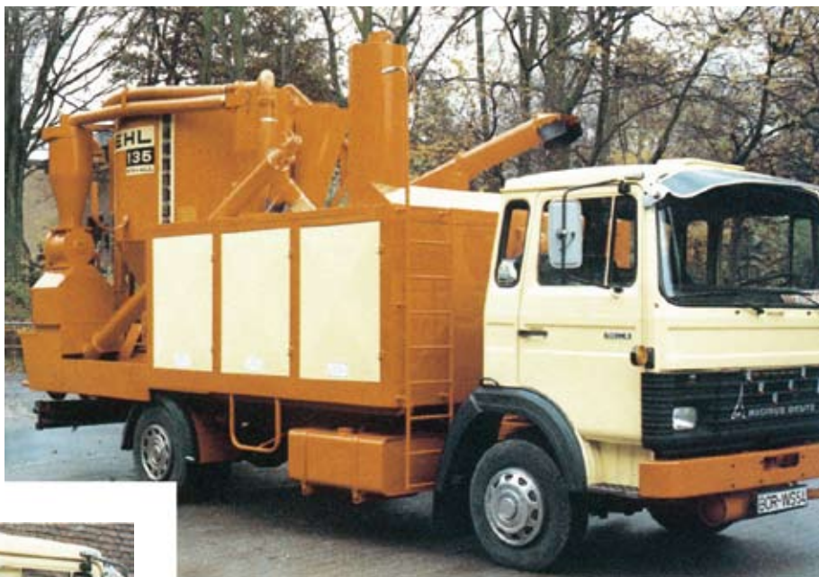
▲ ◀ Aerzen bulk vehicle blower GM 13.f7-1 used on a mobile milling and mixing installation producing feed
