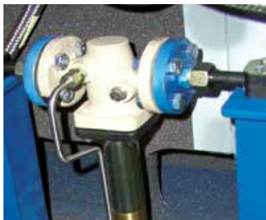
Sealing gas regulator for exhaust compression
