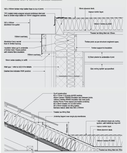
The pitched roof construction consisted of 63x175mm C16 joists at 600 centres. 40mm of Celotex TB4000 insulation was laid between the joists and 140mm of Celotex XR400 insulation was laid over the joists. The roof structure had a Klober Permo Forte vapour permeable underlay, 50x38mm treated sw counter batten and 30x25mm treated sw tiling batten. The tiles for the pitched roof were Samaca natural slate tiles 500x250mm.
