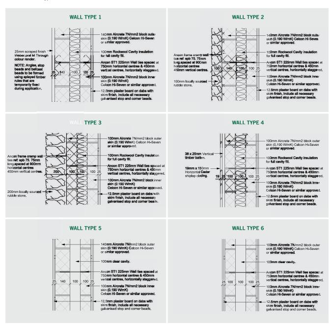
High Strength Grade 440mm x 215mm x 140mm Aircrete 7.3N/mm² blocks were used for the outer skin on wall types 1, 2 and 5.
