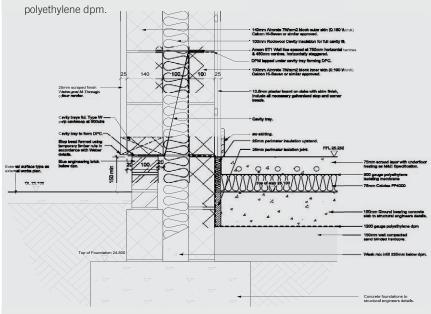
Weak mix infill, 225mm below dpm and then a further 150mm of well compacted sand blinded hardcore was applied directly above the concrete foundations.
