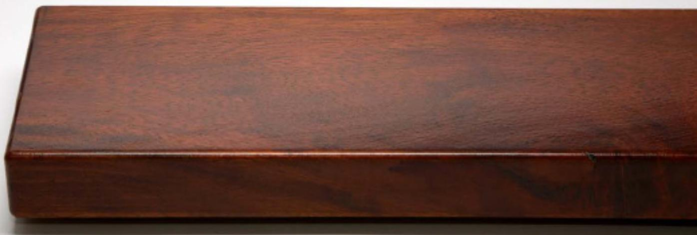
Below shows Iroko timber untreated and freshly sanded. The inset image to the right shows untreated Iroko after seven years exposure and no maintenance. When untreated the timber begins to fade within weeks of being exposed to sunlight. After a time it goes silvery grey. Despite the difference in appearance, the timber remains structurally sound. If desired the surface can be 'cut' back using sand paper to reveal the original colour of the timber.
