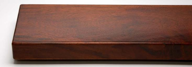
Below shows Iroko timber untreated and freshly sanded. The inset image to the right shows untreated Iroko after seven years exposure and no maintenance. When untreated the timber beings to fade within weeks of being exposed to sunlight. After a time it goes silvery grey. Despite the difference in appearance, the timber remains structurally sound. If desired the surface can be 'cut' back' using sand paper to reveal the original colour of the timber.
