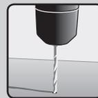
Pre drill holes before installation and oversize any holes by a minimum of 2mm in relation to the size of the fixings.
