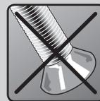
Avoid countersunk screws if possible and do not over tighten. Allow some room for expansion.
