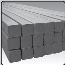
Centriforce recycled plastic profiles can be worked using similar equipment to traditional wood. It can be sawed, and drilled using typical wood working tools or machinery with good results. Circular saws and band saws work well with the profiles, but slower speeds are normally recommended to avoid friction heating and melting. Similarly wood and even metal drills can be utilised, but again slower speeds are suggested.
