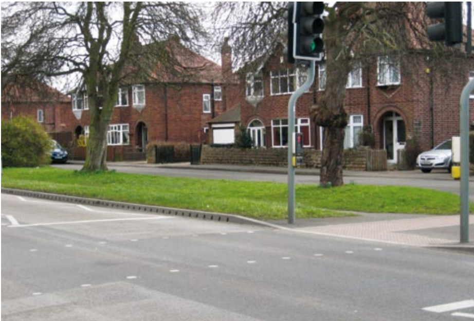
ACO KerbDrain Drop Kerb units allow continuous drainage runs to continue unbroken across road-level pedestrian crossings.
