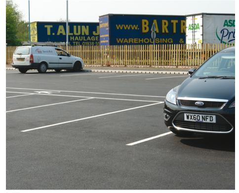
Construction of the extended car park pavement has been greatly simplified with the use of ACO KerbDrain. As run-off can enter at any point along the installed run only a single fall is required.
