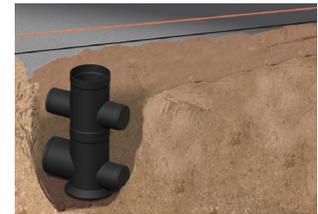
Knock out pre-formed outlet from the inside (marked with hammer symbol) and trim edges with a sharp knife. Fit outlet connector and sump. Position sump and outlet channel on concrete bed, fit PVC-U union/trap to drainage pipework.
