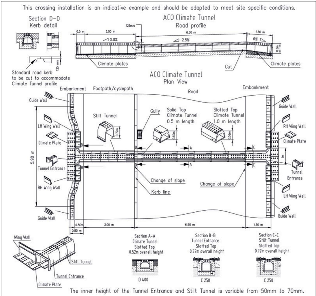
The slotted ACO Climate Tunnel is installed flush with the carriageway, cycle path or verges and adjusted to suit any relevant gradients. The system can be installed in existing roadways by closing one lane at a time. The installation trench has a maximum width of 1000mm and depth of 700mm. The Climate Tunnel system is bedded in concrete in accordance with good practice and the adjacent road surfaces are then repaired.
