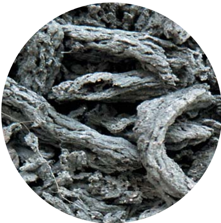
Sludge treated by the BIOCON™ dryer
