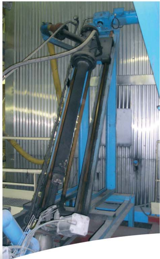
PYROMIX™ injector at Quimper (France) - Injection pipe in raised position
