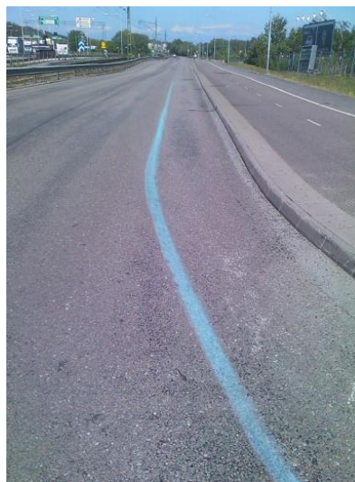
Pictures of a low traffic road in Goteborg/Sweden; Marathon 2010. From left to right: after 3, 6 and 30 days. Colour tone: 1 can AquaRoute® Temp-Paste Blue in 1 bucket AquaRoute® Temp-Base with white pigment.
