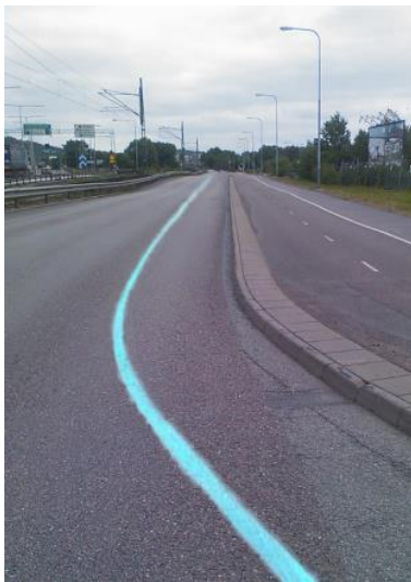
Pictures of a low traffic road in Goteborg/Sweden; Marathon 2010. From left to right: after 3, 6 and 30 days. Colour tone: 1 can AquaRoute® Temp-Paste Blue in 1 bucket AquaRoute® Temp-Base with white pigment.
