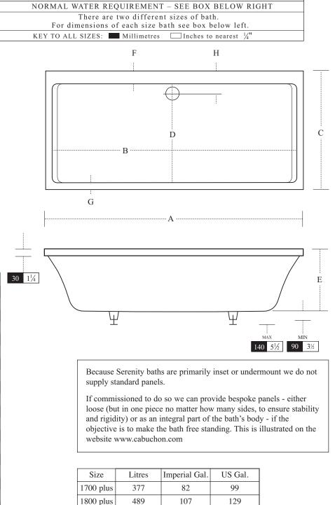
\*Note: On the 1700 Plus the waste/overflow is on the widest rim length. On the 1800 Plus the waste/overflow is on the narrowest rim length.
