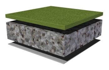
With a unique, porous construction, water drains away ensuring that the area can be used again soon after rain showers. This surfacing can be used to follow nat
