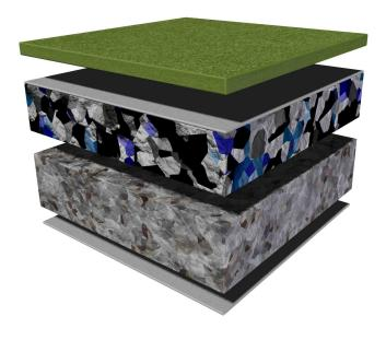
With a unique, porous construction, water drains away ensuring that the area can be used again soon after rain showers. This surfacing can be used to follow nat
