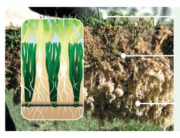
The leaf blades of the natural grass extend above the synthetic grass fibres creating a fully natural grass surface. If the leaf blades are worn away, the sand-dressed synthetic grass fibres continue to provide a consistent, sure-footed playing surface.
