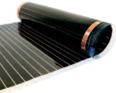
Roydens infloor heating foil is designed to make installation of heating under engineered timber floors even easier. Royden foil comprises of 3 layers of polyester which encapsulates the copper bus bar and conductive heating strips creating an ultra thin heating system in outputs to suit the heating requirements of any building.
