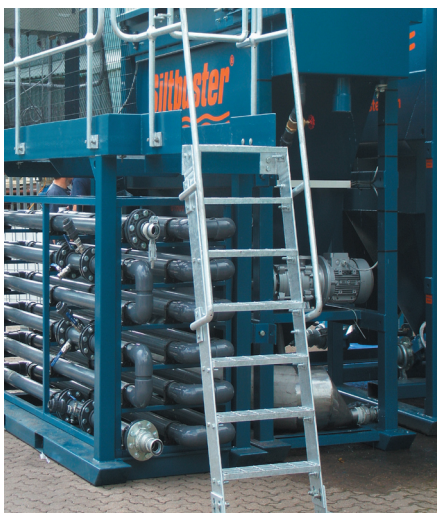
Pipe Flocculator, under access walkway
