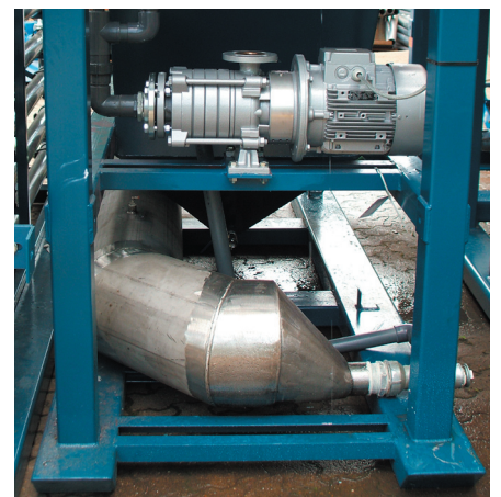
Multi-phase side channel pump and saturation vessel
