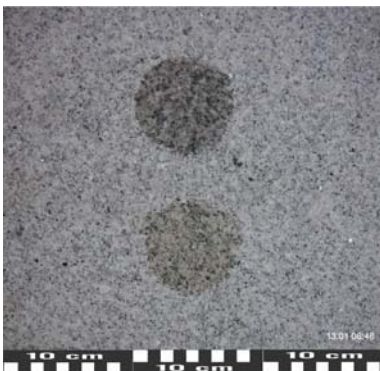
Engine oil and Cooking oil stains on granite
