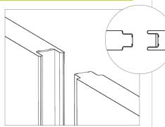
Panels join with a push fit tongue and groove system. Corner posts and T-sections also available.
