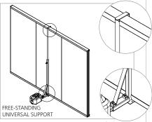
Flamescreen can be installed floor to ceiling using supplied u-channels or for a free-standing system choose our universal support, which can hold 1 - 6 16kg weights.
