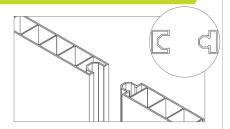
Panels are connected by knocking together the tongue and groove. Corner posts and T-sections are also available to create rooms.
