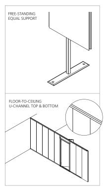
Hoardfast Standard PVC works with a range of free-standing stability options or install floor-to-ceiling supplied u-channels.
