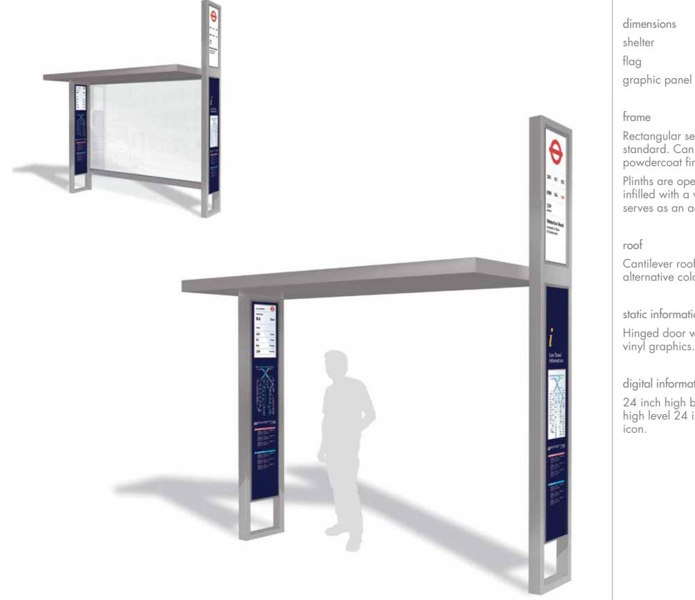
H 3450mm x L 3200mm x D 1250mm H 1000mm x W 350mm H 1900mm x W 350mm
