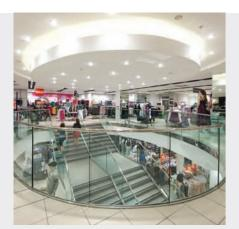
Crystal balustrade in their atrium, a Crystal balustrade with stainless steel handrail on the steps and staircase and an Onyx handrail fixed W Braithwaite to the walls of a second staircase. Mirror-polished Onyx handrails were used throughout. We also manufactured the stairs.
