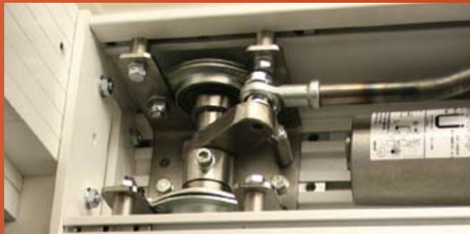
Direct Inhead drive via a standard arm
