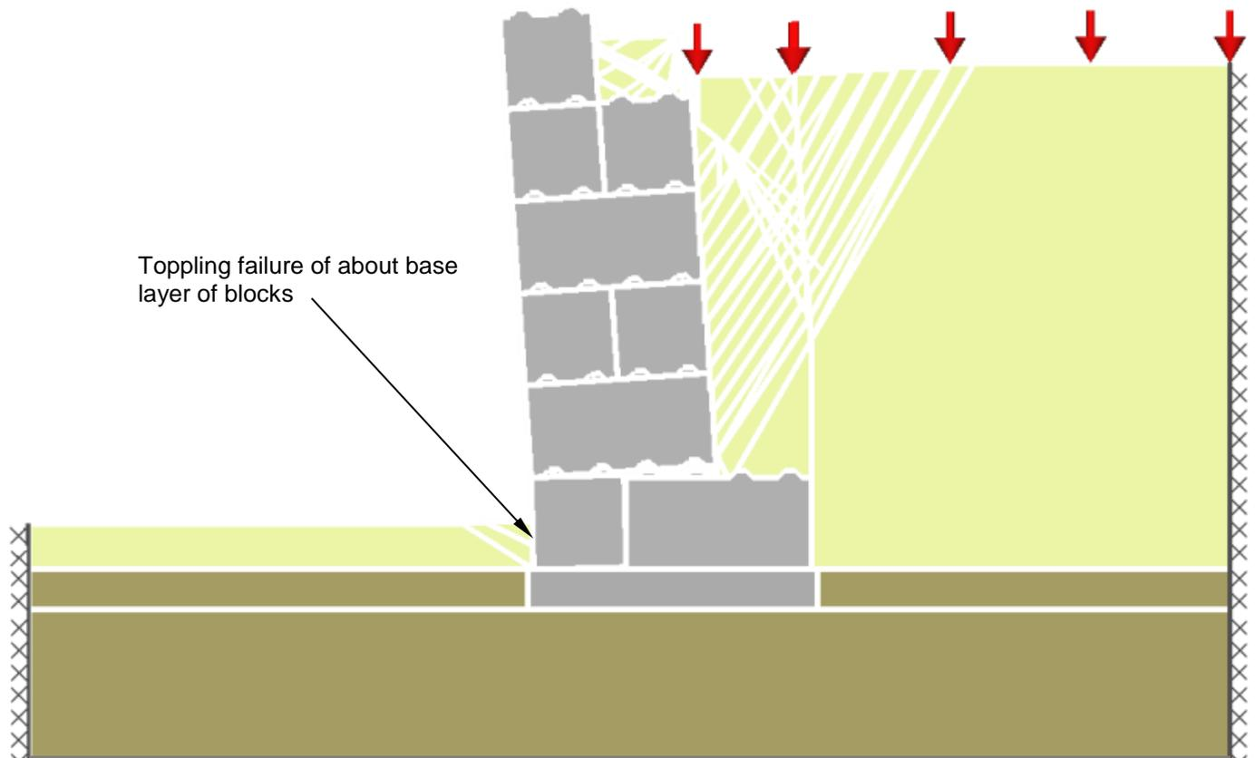
Figure 6.4 Critical failure mechanism through the foundation soil
