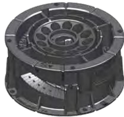
SpiraPave® pedestals are engineered to provide a versatile and cost-effective solution to support raised pavers and timber decking in an eco-friendly way. It provides a cavity for services to be concealed, improves heat and sound insulation and facilitates rapid surface drainage whilst allowing waterproofing and services to remain accessible.
