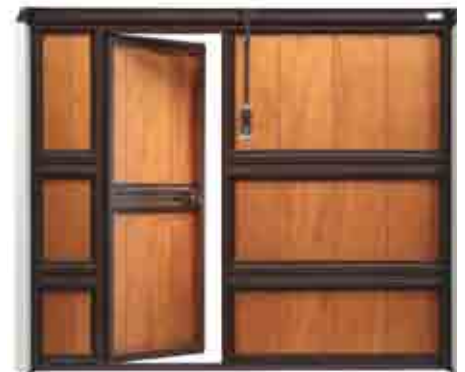
Internal view of Slide with Spazio HF structure and pedestrian door, 90° opening, in tubular perimeter profile in galvanised steel sheet, pressed and painted, and horizontal stiffeners.
