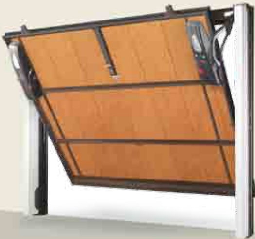
Internal view of Reserve HF and ERG-2 operator, pair of internal pre-fitted internal photocells and pre-wired electrical system (optional). The counterweight sleeves are in pre-painted steel sheet with a white similar to Ral 9016 finish.
