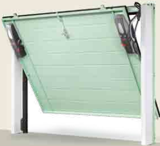
Internal view of Agile up-and-over door with Sikura structure (smooth panel); the Ral 6019 finish, ERG-2 operator, handle art. 98, pair of pre-fitted and pre-wired photocells, are optional. The counterweight sleeves are in pre-painted steel sheet with a white similar to Ral 9016 finish.
