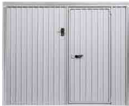
External view of Zink GT with Spazio structure and pedestrian door with 3 locking points, fitted with safety hinge bolts. The pedestrian door, fitted with aluminium hinges and complete with handle and lock, can be side or centrally mounted, according to the size of the up-and-over door.
