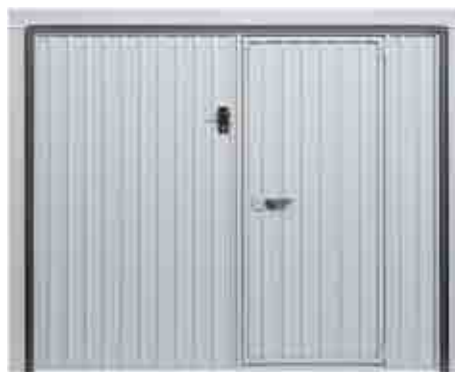
External view of Zink with Sikura HF structure and pedestrian door with 3 locking points. The pedestrian door, fitted with aluminium hinges and complete with handle and lock, can be side or centrally mounted, according to the size of the up-and-over door.
