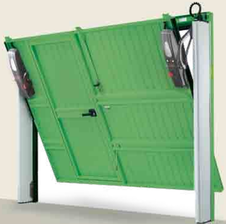
Internal view of Zink GT up-and-over door with Spazio HF structure and perimeter seals. The pedestrian door, ERG-2 drive with pre-fitted internal photocells, pre-wired electrical system, and RAL 6018 finish are optional. The counterweight sleeves are in pre-painted white- grey steel sheet.
