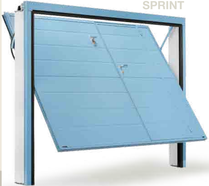
External view of Sprint up-and-over door with Spazio HF structure, external side with smooth panel (pitch 250 mm) and internal side with multi-line panel. The pedestrian door and the Ral 5024 paint finish are optional.
