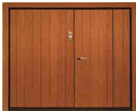
External view of Reserve HF with pedestrian door incorporated in the mobile leaf. 90° opening Pedestrian door in tubular perimeter profile in steel sheet, galvanised and painted, and horizontal stiffeners. Equipped with steel hinges, totally concealed, and 3-point locking with double map key to guarantee improved safety against intrusion.
