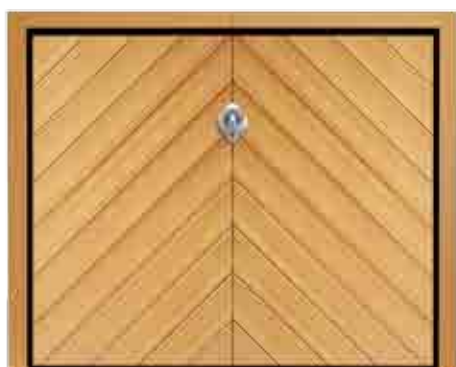
Special HF model with herringbone slats, pitch 192 mm, 45° angle pointing upwards. External cladding thickness 15 mm, available in Okoumè ply, or Okoumè ply with external veneer in Oak or Douglas Pine. Alternatively they are available in Fir or Larch, both laminated and with exposed knots, also with a brushed finish. Total thickness of mobile leaf: 105 mm.
