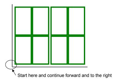
Take next panel of pavers, correctly orientate, line up edge with first panel and apply foot pressure to complete connection. Continue laying panels ahead and to the right. If required pavers can be easily cut with a saw. Should it be necessary to separate individual pavers from panels, apply foot pressure to left side pavers and pull up right side pavers from the bottom, i.e. 'unzip' pavers.
